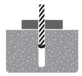
With the correct diameter drill bit, drill a hole to the correct depth
